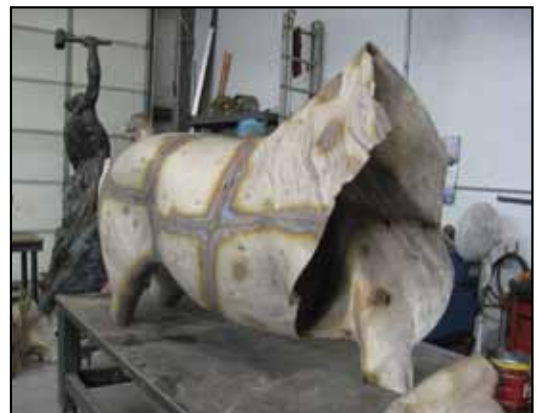
Grinding the weld lines of the bronze to recreate the texture of the original clay sculpture. Fifty-one metal panels and parts are welded together.
